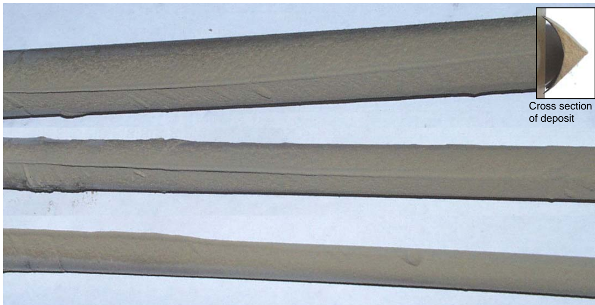
Fig. 37: View at windward side of test tubes (d10, d15, d21) with deposits
